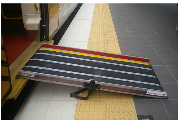
Figure 77 Boarding ramp at low level platform, Roma Street station
