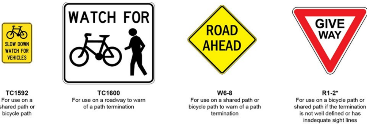
Figure C.9 – Signs used for slowing people riding bikes and warning of a path termination
